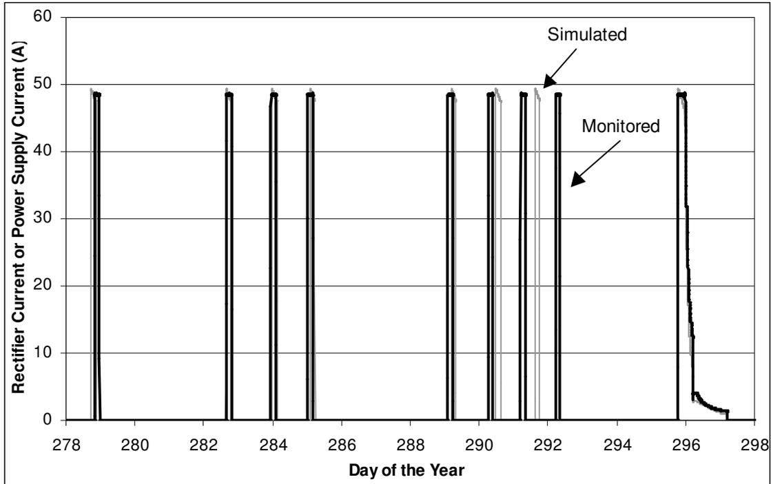
**Figure 9:** Rectifier Output—Measured versus Simulated, PV Hybrid Test #1
