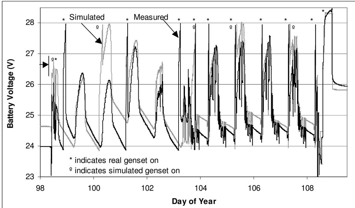
**Figure 14:** Battery Voltage during Second Half of PV Hybrid Test #3
