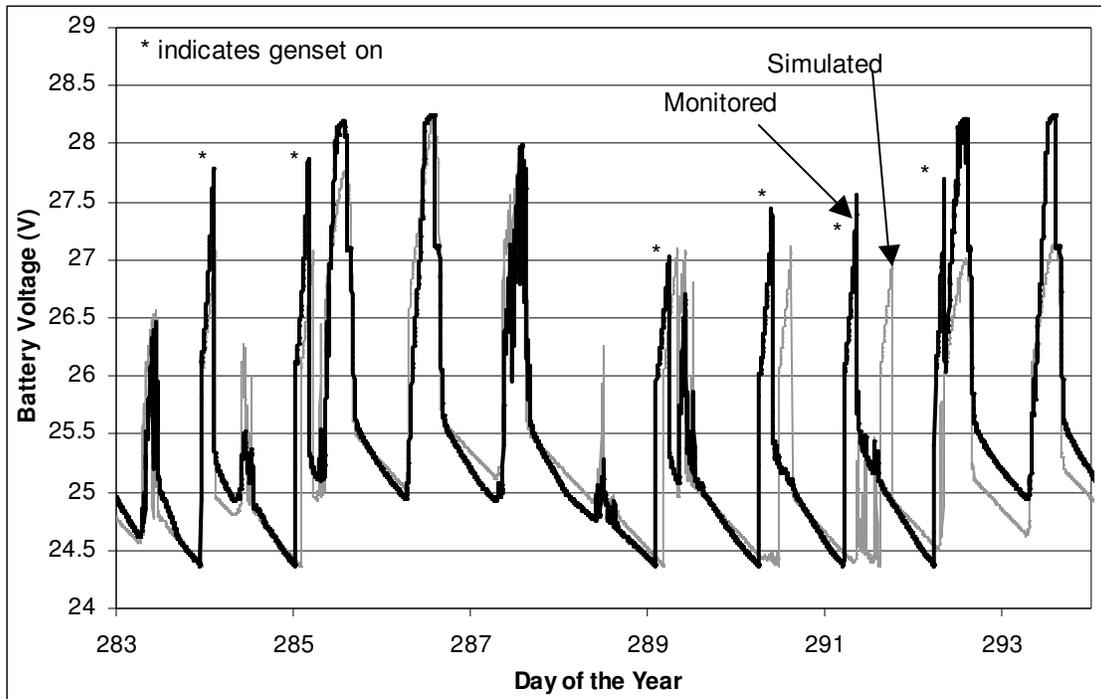
**Figure 10:** Simulated and Measured Battery Voltage, Days 283 to 294, PV Hybrid Test #1
