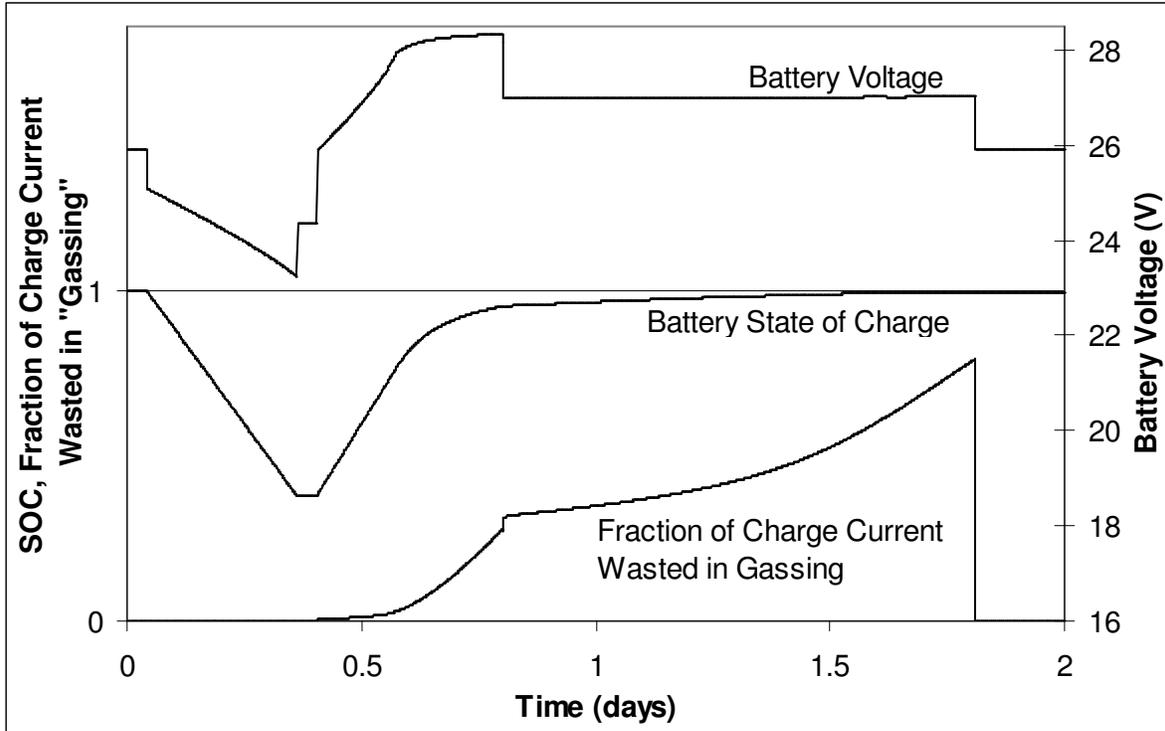
**Figure 2:** Simulated Battery Voltage, State-of-Charge and Gassing Losses during Discharge/Charge Test
