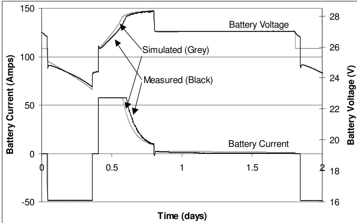
**Figure 1:** Monitored and Simulated Battery Voltage and Current during Discharge/Charge Test
