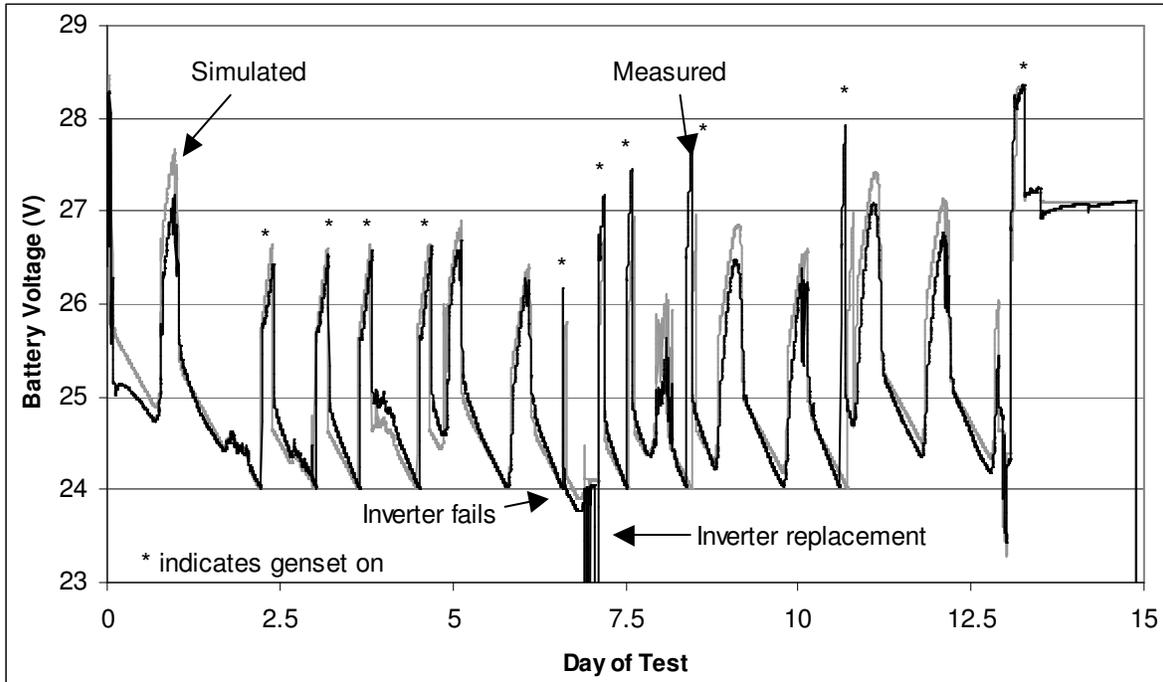
**Figure 11:** Battery Voltage During the PV Hybrid Test #2
