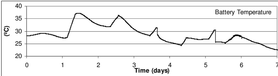
**Figure 3:** Battery Temperature during “Battery Cycling without Absorb Charging” Test
