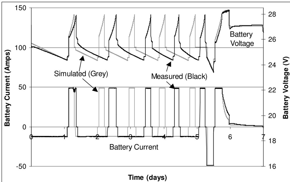
**Figure 6:** Reality vs. Simulation Using Voltage Setpoints
