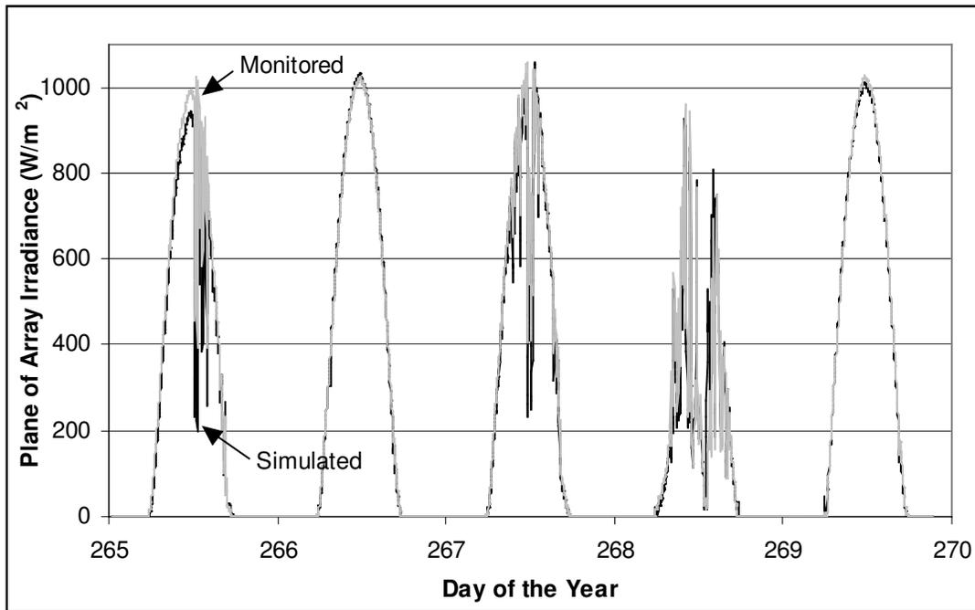
**Figure 8 :** Plane of Array Irradiance—Measured versus Simulated, 2 Minute Data
