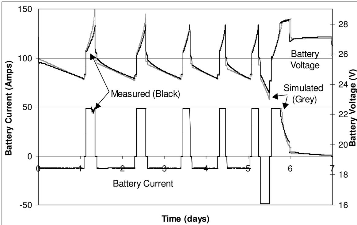
**Figure 4:** Reality vs. Simulation Using Measured Battery Current
