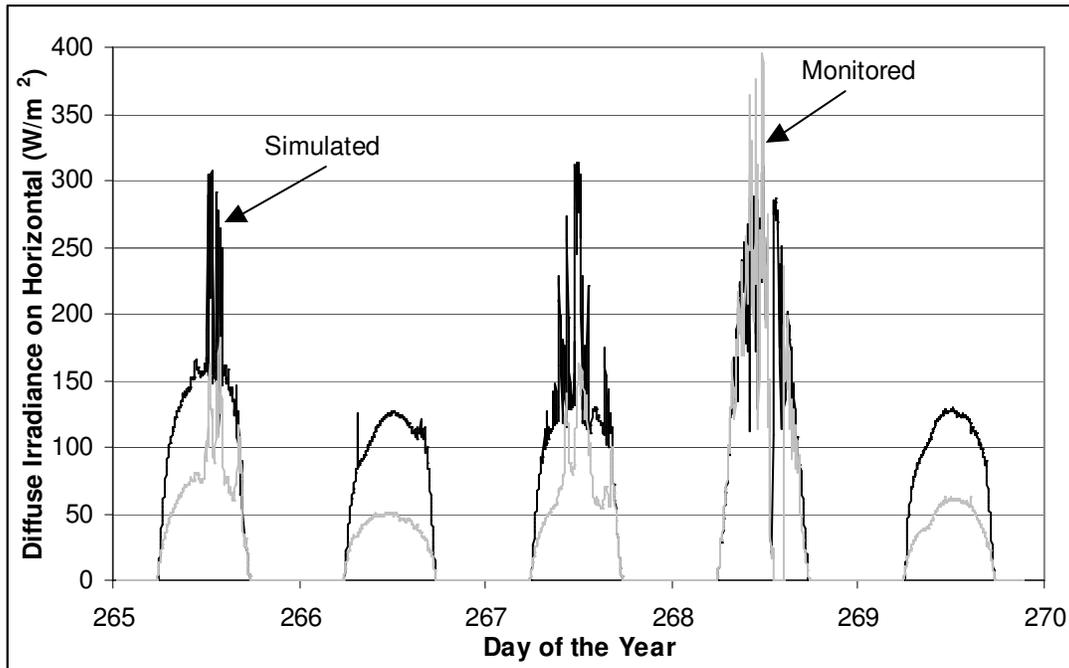
**Figure 15:** Measured and Simulated Diffuse Irradiance on Horizontal, Five days from PV Hybrid Test #1
